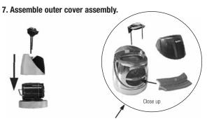
Note. Verify that rubber insert is installed
